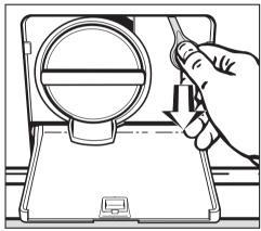
■ Pull the emergency release downwards (see illustration). The drum door will open.
